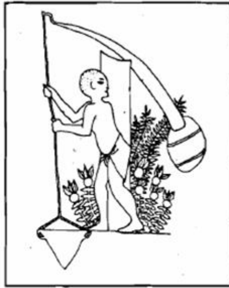
Fig. 1.13 An Egyptian farmer lifting water by lowering a cone-shaped leather bucket which hangs from a beam, balanced across a pillar. The weight at the other end helps the farmer to lift the filled bucket with less effort. Sketch from a tomb painting about 1500 B.C. In India, even today such a device called 'dhenkli' is used.
